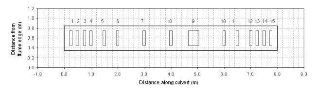
Figure 1. Plan view of culvert showing location and size of culvert access holes.
