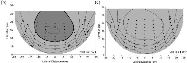
Figure 6. Distribution of Vx non-dimensionalized with respect to  $V_{mean}$  at hole 14 for a discharge of 70 L/s and: (a) tailwater depth set at normal depth, (b) tailwater depth set at 4.4 cm above normal depth, and (c) tailwater set at 6.4 cm above normal depth.
