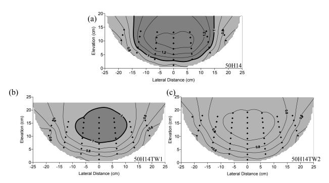
Figure 5. Distribution of Vx non-dimensionalized with respect to  $V_{mean}$  at hole 14 for a discharge of 50 L/s and: (a) tailwater depth set at normal depth, (b) tailwater depth set at 4.4 cm above normal depth, and (c) tailwater set at 6.4 cm above normal depth.
