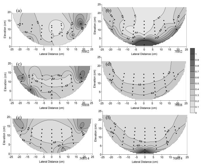
Figure 7. Distribution of  $I_{mag}$  for (a) 50 L/s at hole 2, (b) 70 L/s at hole 2, (c) 50L/s at hole 8, (d) 70 L/s at hole 8, (e) 50 L/s at hole 14, and (f) 70 L/s at hole 14.
