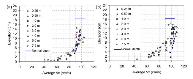
Figure 4. Centerline vertical velocity profiles for (a) 50 L/s and (b) 70 L/s.
