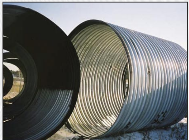
CSP WITH SCREW JACKS AND GROUT PLUGS
