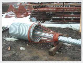
CONICAL GRATE WITH PERFORATED CSP
